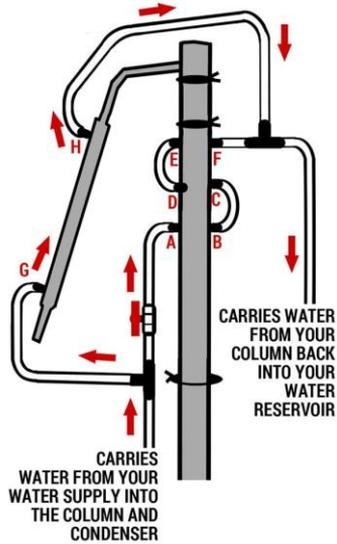
**Attaching the Hoses with the Water Control System:**
